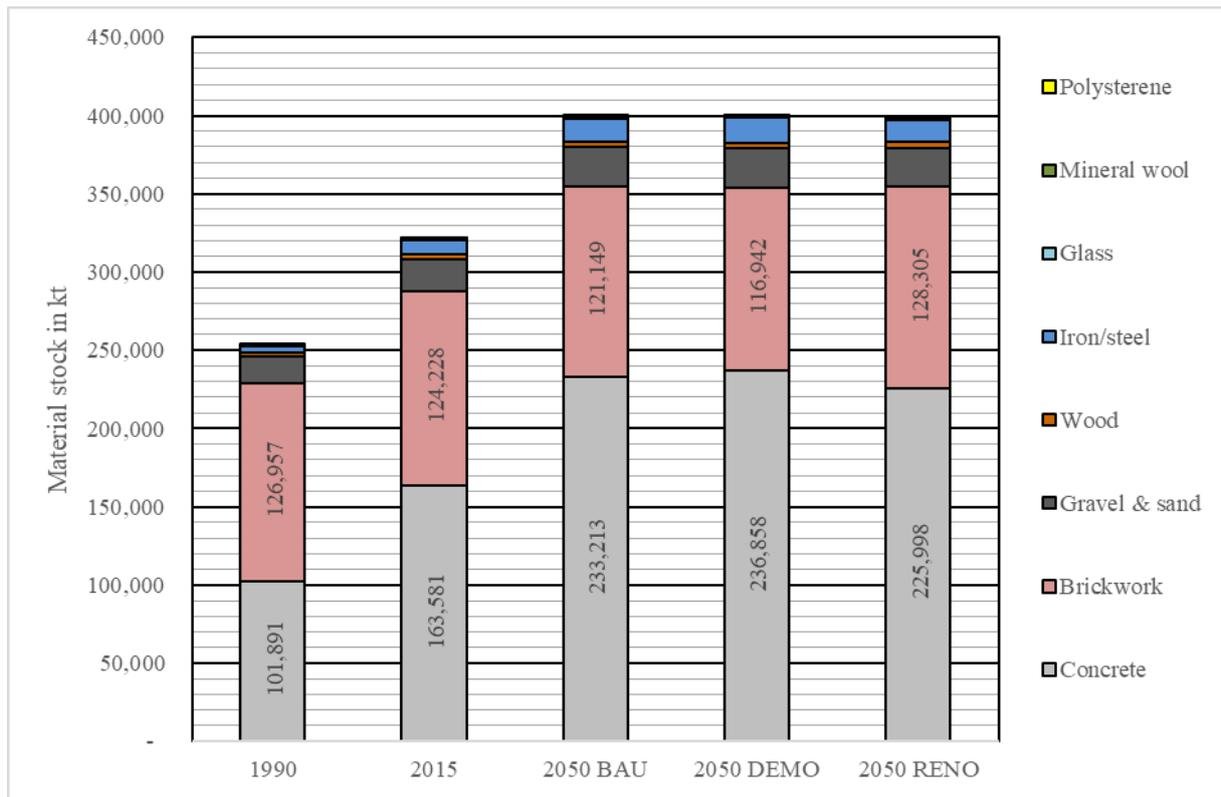
**Figure 15 Construction material stock for the building sector in scenarios developed in [7]**
