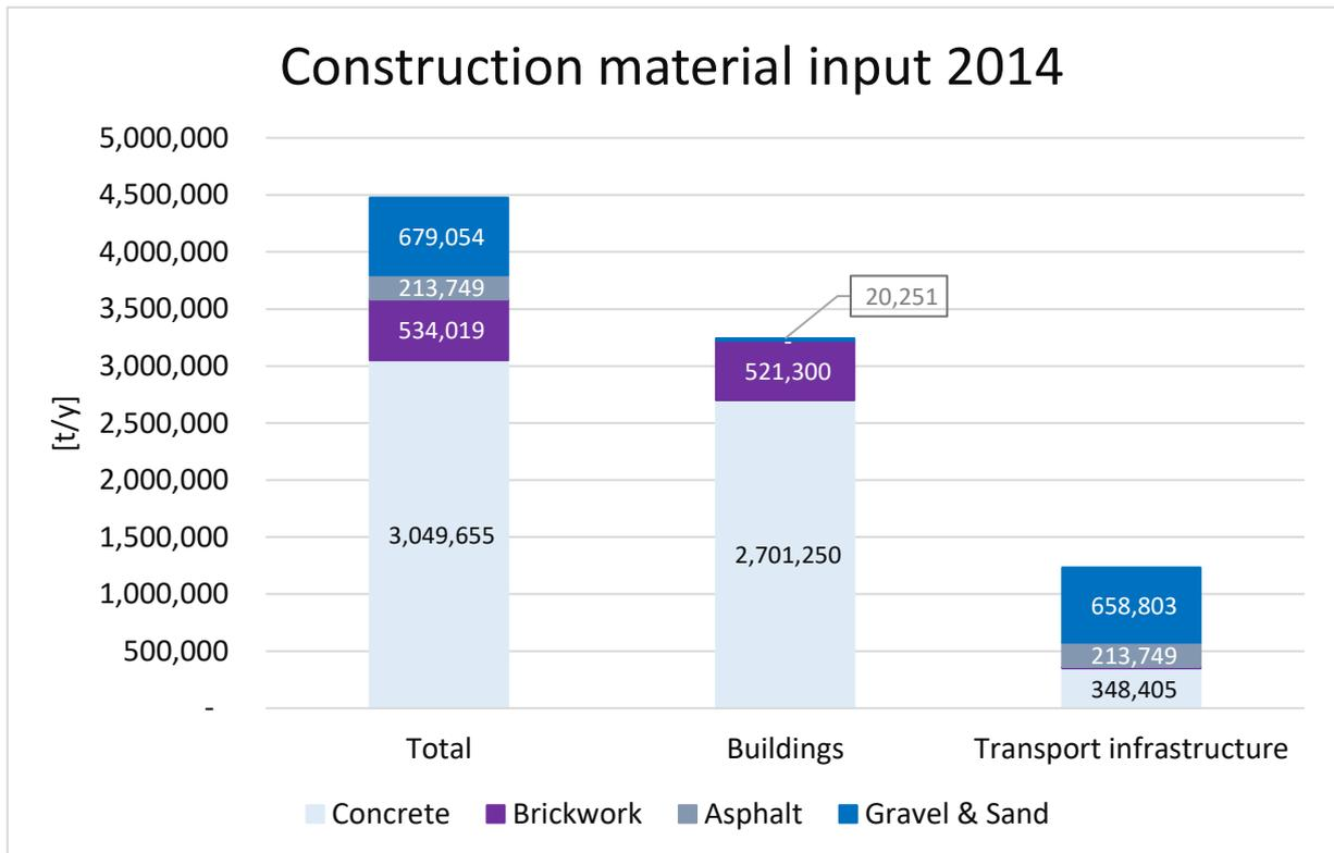
**Figure 18 Construction material inputs for the building and transport sector in Vienna 2014** [17]
