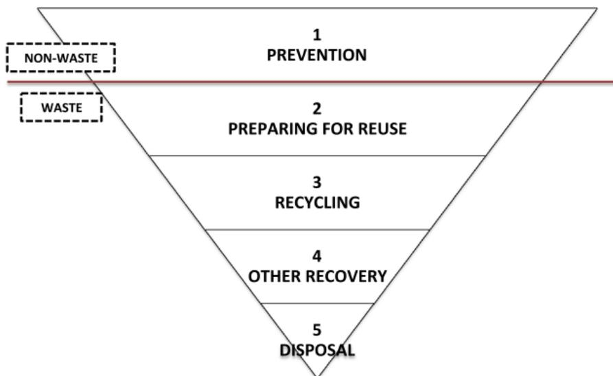
**Figure 1 Waste hierarchy according to WFD2008, image from [22]**
