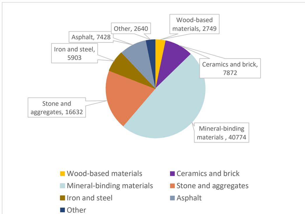
**Figure 11: Construction material stocks per material type in Gothenburg in ktons (2016) (Source: [79])**
